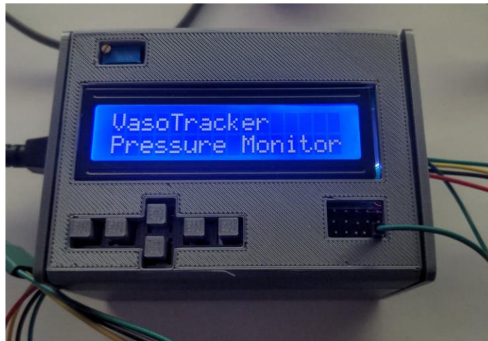
Figure 13 – A programmed pressure monitor.
