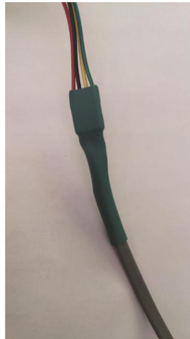
Figure 5 – Pressure sensor connections before (Step 3) and after (step 4) being secured with heat shrink tubing.
